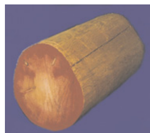
Boron diffusion shown via curcumin test after 4 months at approx. 85% humidity.
